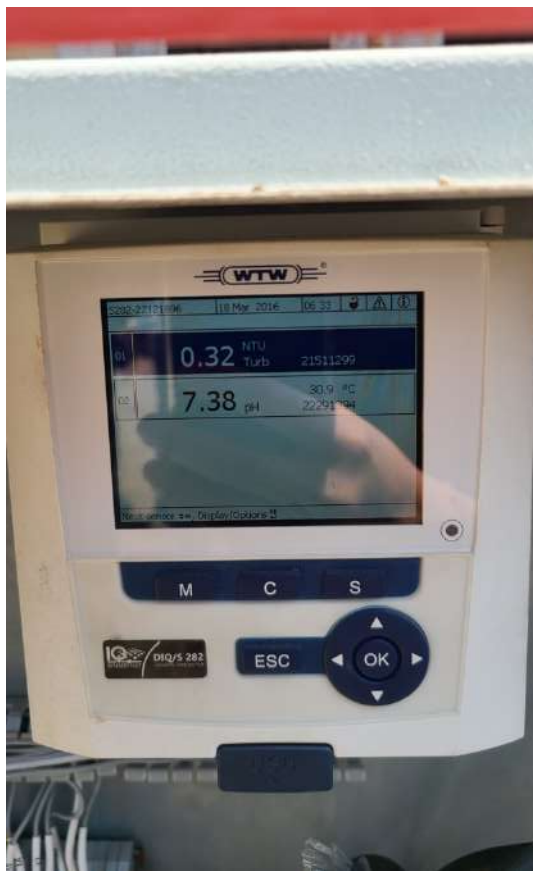
Figure 36: Ultrasonic Flowmeter reading (left), Turbidity and pH sensor at WTP (right)
